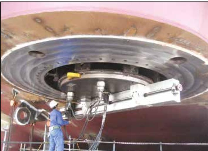
▼ Machining crane bearing face.
