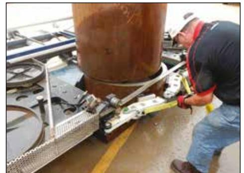
▲ Pipe cutting with Mirage BS portable band saw.
