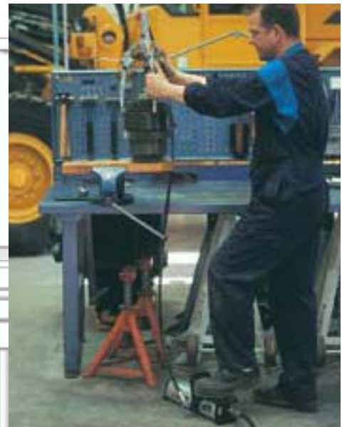
Express puller EP55 in three-arm-mode operated by air/hydraulic pump PP70-1000
