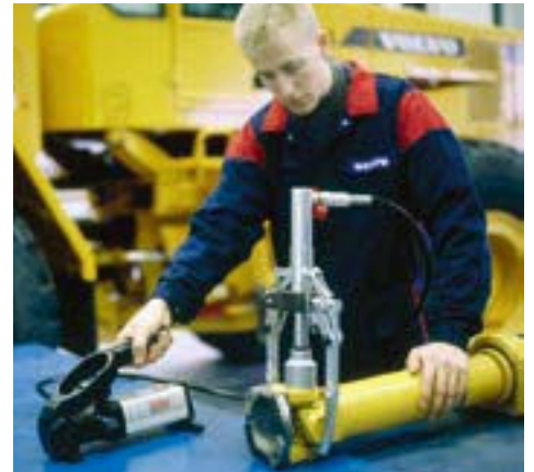
Converted two arm express puller EP55 operated by hydraulic hand pump
