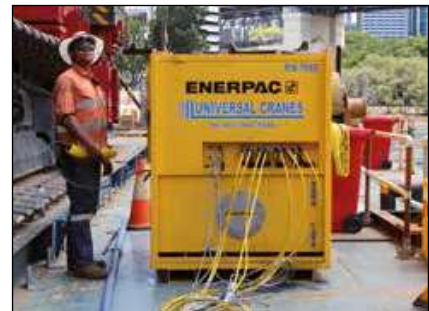
▼ SyncHoist Powerpack to operate the 4 lifting points.
